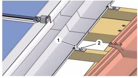
Fig. 18: Fixing for flashing on flashing sides
