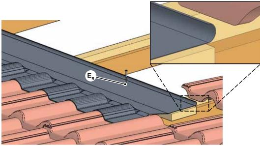
Fig. 31: Lead flashing on roof slopes <22°
