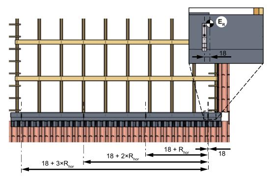
Fig. 32: Mounting clamps horizontal positions
