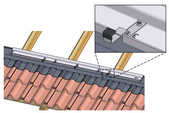
Fig. 35: Place Mounting Clamps Glass
