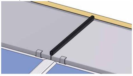
Fig. 60: Mounting protective profile
