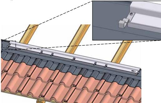
Fig. 34: Fitting the mounting gauge
