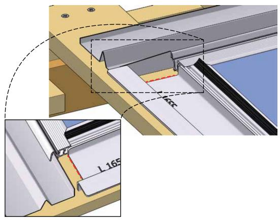
Fig. 46: Aligning the mounting clamp
