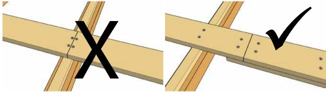
Fig. 66: Incorrect / correct joints
