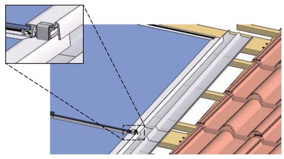
Fig. 50: Lay remaining modules
