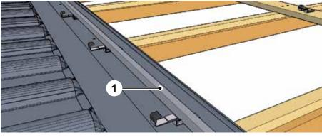
Fig. 16: Sealing tape strip
