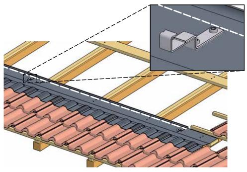
Fig. 33: Mounting clamps bottom row
