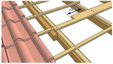
Fig. 65: Cutting a batten to size
