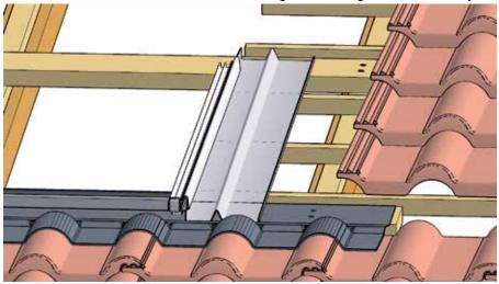
Fig. 38: Flashing profile right
