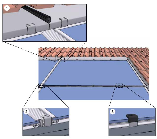
Fig. 9: Mounting clamps mounted
