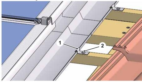
Fig. 61: Fixing for flashing on flashing sides
