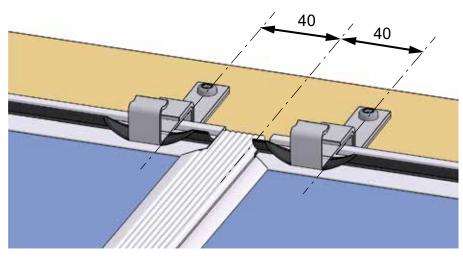
Fig. 52: Mounting clamps top row transitions
