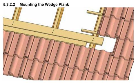
Fig. 28: Mounting the wedge plank
