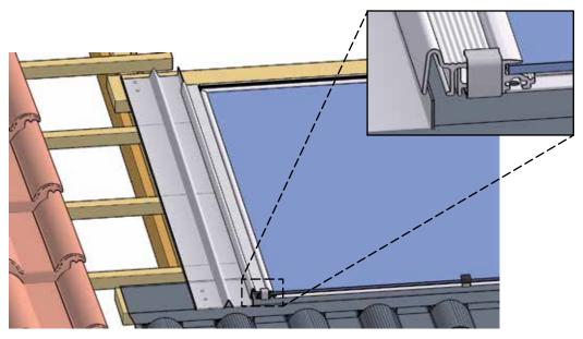
Fig. 42: Inserting flashing profile left
