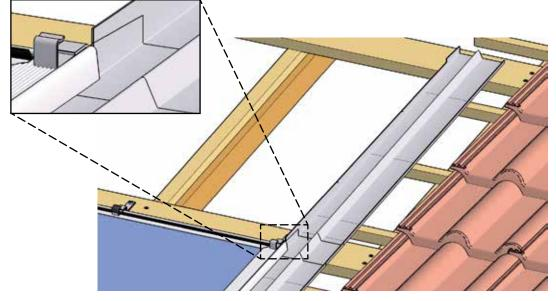
Fig. 48: Push in flashing side right
