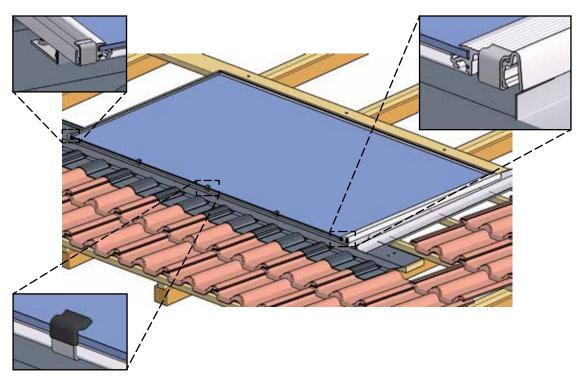
Fig. 39: Lay the first module
