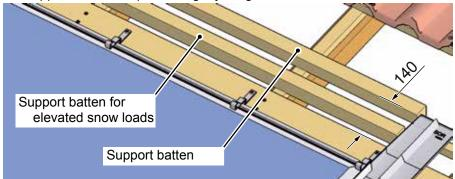
Fig. 56: Support battens
