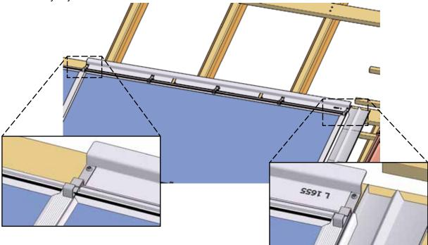
Fig. 47: Mounting the remaining mounting clamps
