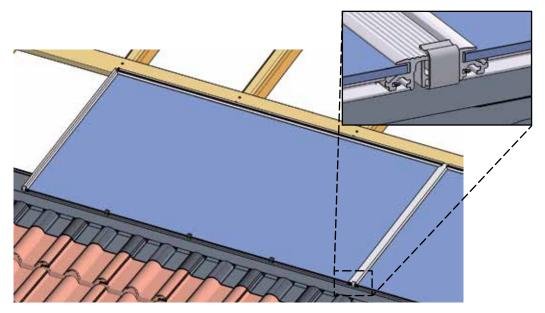
Fig. 40: Lay remaining modules
