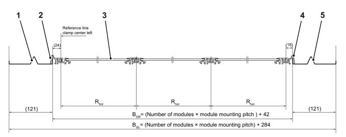
Fig. 5: Horizontal cross-section
