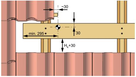
Fig. 26: Mounting the bottom Solrif® batten
