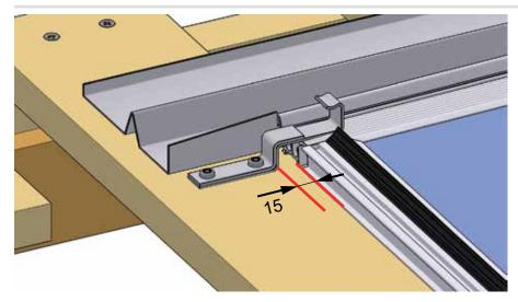
Fig. 43: Mounting clamp distance
