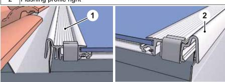
Fig. 11: Flashing profiles mounted
