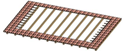
Fig. 23: Removed tiling battens
