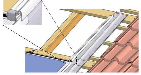
Fig. 49: Push in the flashing profile right
