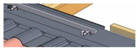
Fig. 36: Laying the sealing tape strip
