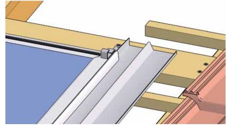
Fig. 51: Mounting clamps top row edge
