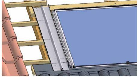
Fig. 41: Laying flashing side left
