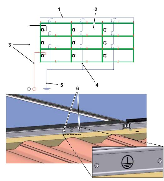
Fig. 17: Drilling work for grounding
